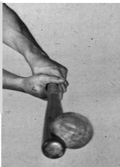
The collision of a ball with a bat collapses part of the ball.
